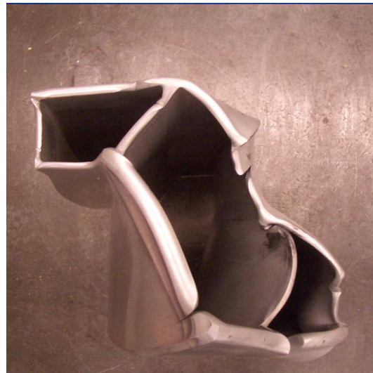
Figure 9: head of the extruded profile after the first trial at the press.
